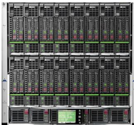
HP C7000 Chassis Enclosure
